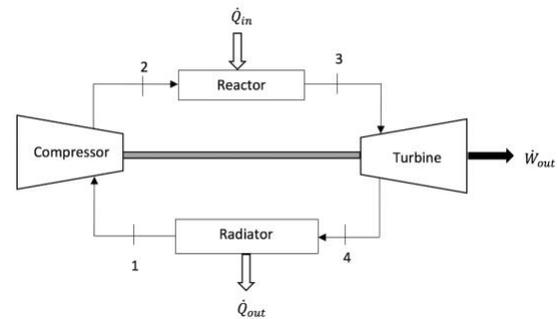
Fig. 2. Closed-loop Brayton Cycle Schematic [8]
