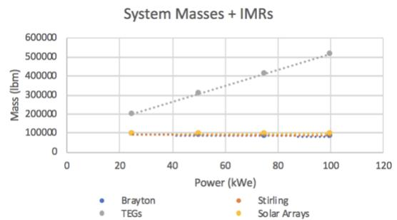
Figure 12. Design A System Masses plus IMRs vs Power
