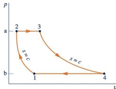
Fig. 3. Closed-loop Brayton Cycle Pressure vs Volume
