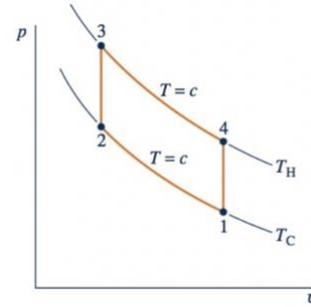
Fig. 7. Stirling Cycle Pressure vs Volume
