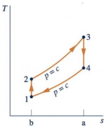
Fig. 4. Closed-loop Brayton Cycle
