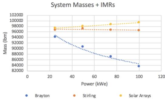
Figure 13. Design A System Masses + IMRs vs Power without TEGs
