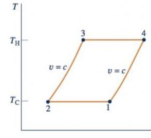
Fig. 8. Stirling Cycle Temperature vs Entropy
