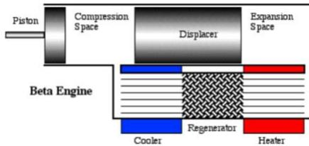
Fig. 6. Beta Stirling Engine Schematic
