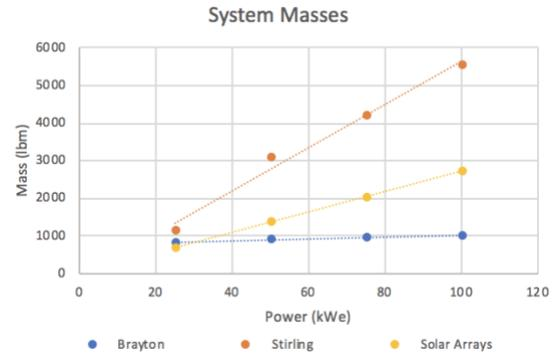
Figure 11. Design A System Masses vs Power without TEGs
