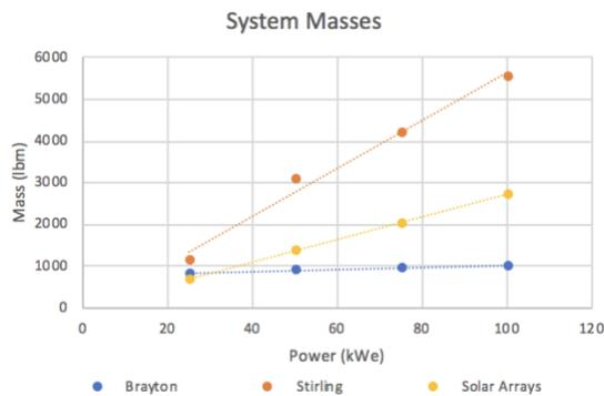
Figure 14. Design B System Masses vs Power
